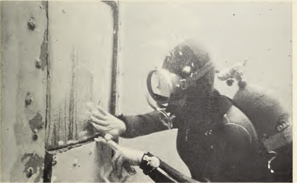
This diver sheepishly admitted attempting to wipe the window clear from outside. A wetting agent is used to keep the windows clear of fogging.
